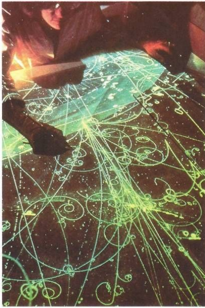
Tracks made by atomic particles from a particle accelerator, a device that speeds up the particles, are recorded on film. Physicists study the tracks to learn about the characteristics of the particles that produced them.
